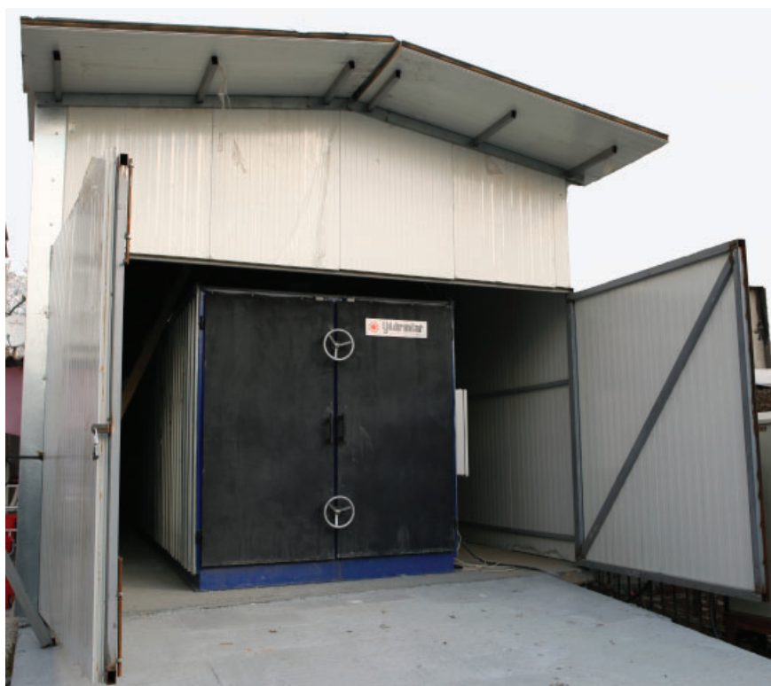
Fig. 8b. A 10 m long drying oven for large-scale timbers at Yenikapı Site Lab.
