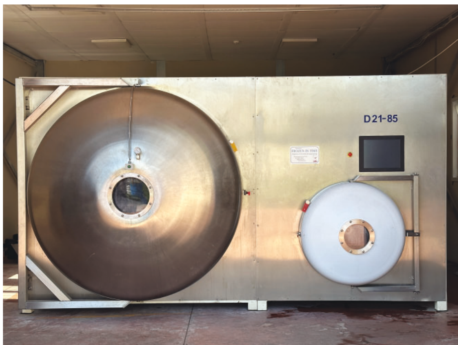
Fig. 7a, b. D 21/85 model vacuum freeze dryer used in the Yenikapı Shipwrecks Project.
