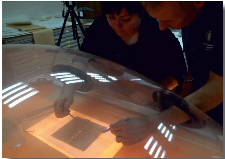
Fig. 1.4. Restorers Mymrina Ye. V. and Prokhorov R. Yu. during working in the remote humidification chamber
