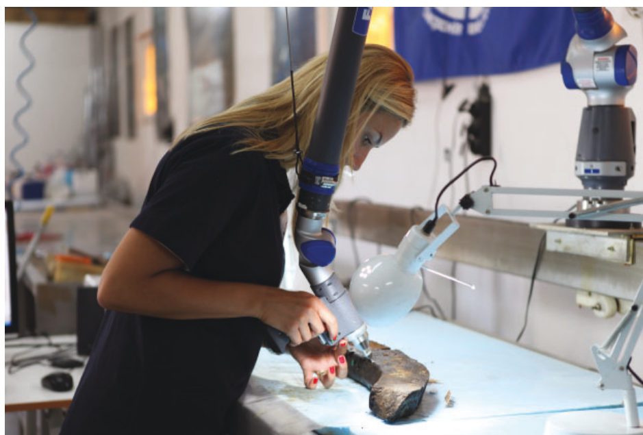
Fig. 5. 1:1 scale digital drawings with the digitizer (FaroArm) device.
