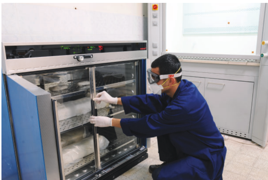
Fig. 8a. Placing the small timbers of the shipwrecks in the drying oven (Yenikapı Site Lab.)
